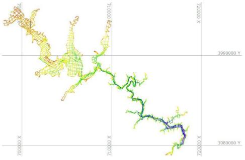
Figure 5-6. Track line locations for the bathymetric and sediment depth survey Color is shown to provide a visual interpretation of water depth.
